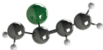
Neoprene (CR) rubbers are homopolymers of chloroprene (chlorobutadiene), and were among the earliest synthetic rubbers used to produce seals. CR has good ageing characteristics in ozone and weather environments, along with abrasion and flex-cracking resistance.
