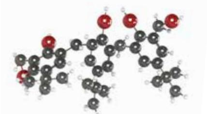
Phenolic resins, also known as phenol formaldehyde resins (PF), are synthetic thermosetting materials created by the reaction of phenols with formaldehyde. These thermosets perform well in most engineering applications such as: hydraulic fluids, oil, glycols, phosphate esters etc.
