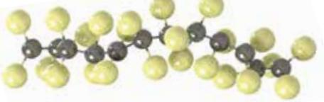
PTFE (polytetrafluoroethylene) is a synthetic, thermoplastic polymer and offers exceptional chemical resistance over a wide range of temperatures, as well as extremely low levels of friction.
