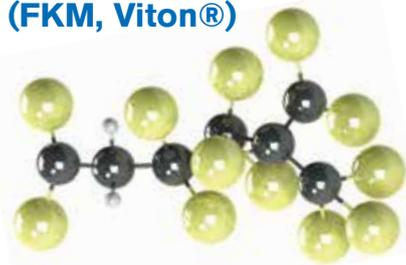
FKMs (sometimes known as FPMs in Europe) are frequently used to resist extreme temperatures and harsh chemicals. The strong carbon-fluorine bonds that make up the polymer structure provide high thermo-chemical resistance, giving excellent ageing characteristics shown by low compression set at elevated temperatures.
