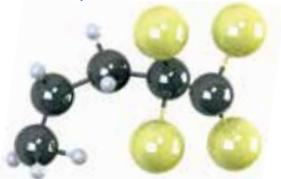
The most common forms of Aflas® (100 or 150 series) are categorized within ASTM D 1418-01 as FEPM. These grades are alternating copolymers of tetrafluoroethylene and propylene, with a fluorine content of ~54%. Such chemical structures offer excellent heat resistance, exceptional chemical resistance (significantly to alkalis and amines), along with high electrical resistivity.
