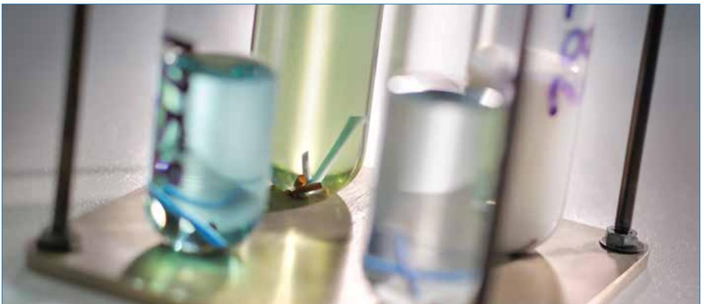
*Chemical immersion test/wet bench analysis.*
