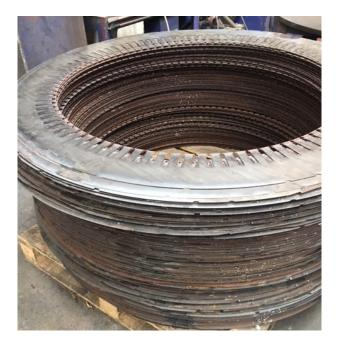
Once the outer case end was removed, the core pack was secured in place, while the welds on the support struts were also removed along the entire length of the core. A keyway was then manufactured and fitted, preventing the core from moving, maintaining its skew.
