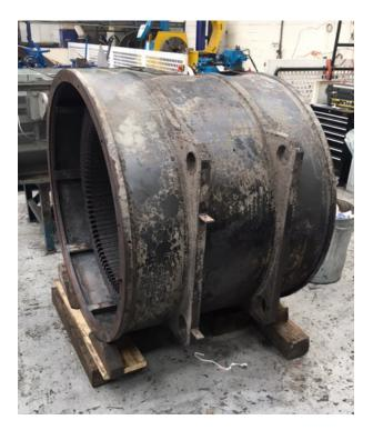
Several internal meetings were held, and a solid repair programme was created, which included the construction of various specialised jigs that would enable the support of the core and keep a mechanical datum.
