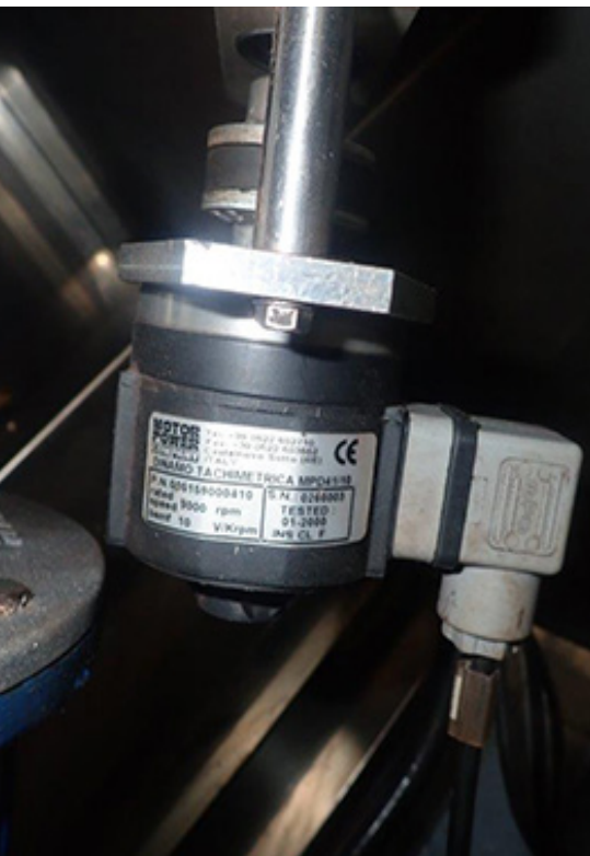
Tachometer fitted to input shaft
