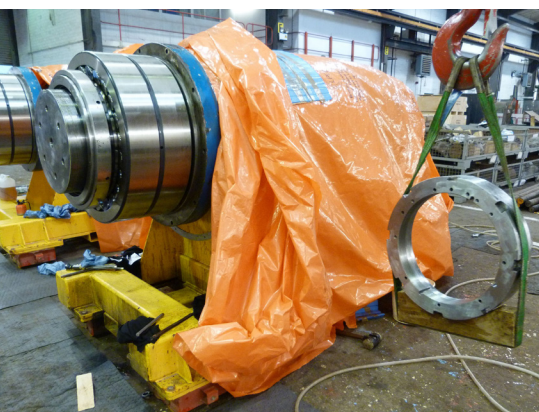
Mounting the hydraulic nut onto the shaft
