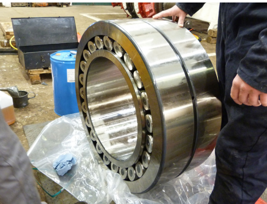
Inspecting the bearing for damage
